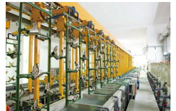
Automatic plating lines to ensure the stability of ELUS stunning chrome finish along with other colorful surface finishes such as brushed nickel, matt black, luxury gold, and oil-rubbed bronze.
