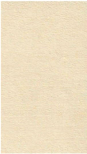
Plaster brown 配比: 4g F01 /10kg microcement
