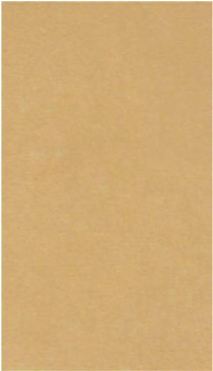
Plaster brown 配比: 50g F01 /10kg microcement
